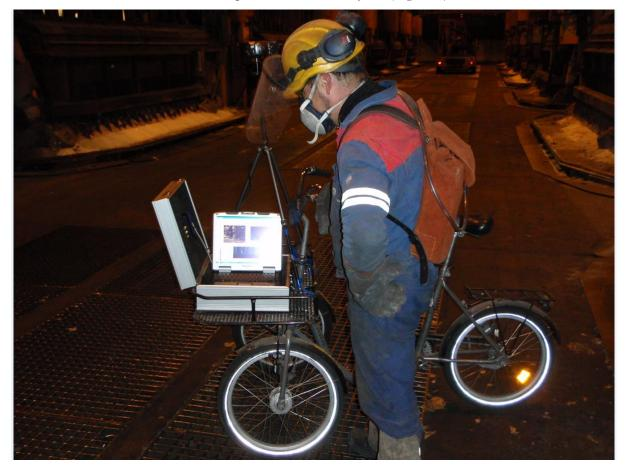
A steady backpack, to be carried by the studied worker, for the monitoring instrument and the transmitter is necessary. Because of strict rules on use of inflammable material in this industrial branch, a specially manufactured backpack, e.g. in leather, must be used. An example from one factory is showed in figure 3.
